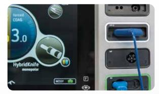
The active slot and the instrument in use are shown on the display and through the illuminated socket frame.
