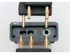
Standard instruments can be inserted into any universal socket.
