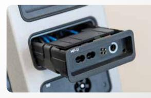
Sockets can easily be replaced without opening the casing.
