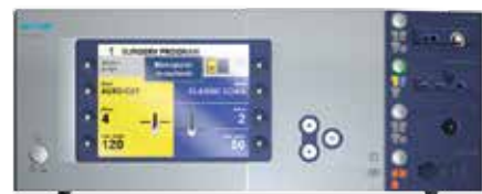
VIO electrosurgical unit with display for CUT and COAG settings
